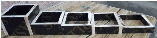
Figure 1. Mold used for pouring concrete.
